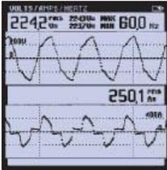
Figure 10C. Flat-topped waveforms
