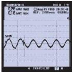
Figure 9A. Overvoltage transient capture.
