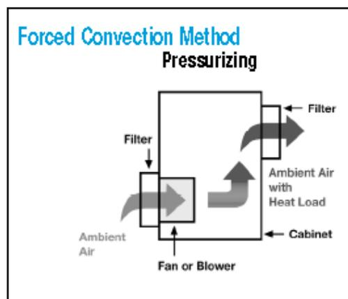
The Pressurizing Forced Convection Method( on right above) is preferred in that only air filtered by the fan flows into the switch cabinet.
