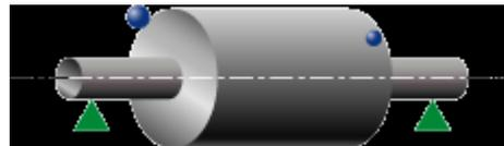
When the part rotates it generates centrifugal forces. Normally, the sum of these centrifugal forces equals zero, however, if they do not, that rotating object will generate vibration and noise. Dynamic balancing machines (as shown on left) measure the amount and angle of this vibration.
