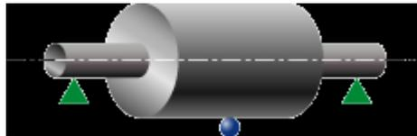
Static Balancing is a weighting process to detect the imbalance of a circular or cylindrical part which is free to turn on an axis. A part to be balanced is placed on the four discs of the Balancing Tool. An unbalanced part will rotate until the heavy side is downward. Balance is accomplished by adding a counter weight to the lighter side, or by removing weight from the heavy side. When the part remains motionless when placed in any position in 360 degrees, it is then in static balance.
