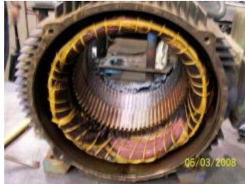
Here we see what happened at the opposite end of the motor. No grease here on winding, same with rotor
