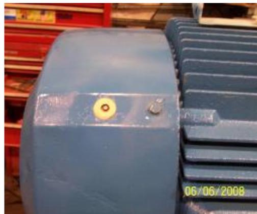
Shown on the left is the plastic plug covering the grease fitting, on the right is our mod to show the grease fitting. The original grease fitting was about 2" below the fan cover plug, we extended it out to be flush.
