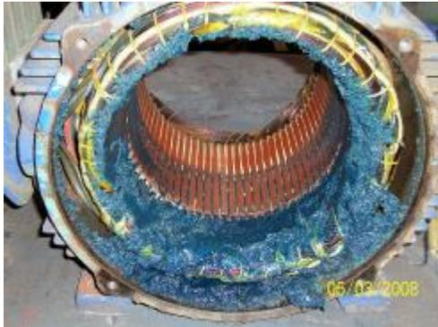
Above and below we see what happened at the motor shaft end of the motor. Much too much grease here. Led to motor winding shorting out.
