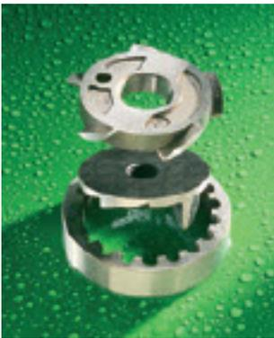
As an example Hydromatic Grinders use an exclusive “dual cutter” design that prevents clogging, binding, and roping in a wide range of operating conditions. These cutters cut waste twice to reduce it to an even finer slurry. The first cut is performed by the radial cutter; the second by the axial cutter that “recuts” the waste in a perpendicular direction to the radial cutters. This creates even smaller-particles, making for better sewage flow.
