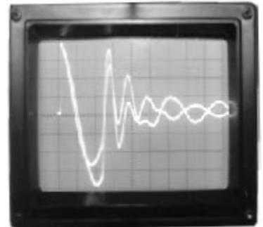
**Faulty Comparison Patterns.** Waveforms are erratic during the test (left) or separated throughout the entire trace (right).
