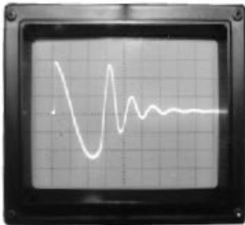
**Good Comparison Pattern.** Only one wave appears on the surge tester screen when two tests are displayed simultaneously. (The wave patterns being compared are superimposed exactly.)
