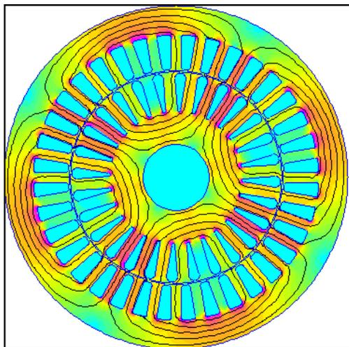
The picture to the left shows a representation of the magnetic flux inside a 4-pole induction motor.
