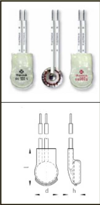
Thermik's S05 style thermal protectors, with normally closed contacts and with an insulating housing, can be used in most environments. This small device has a maximum switching current of 10 amps and temperatures ranging from a low 50°C up to 180°C in 50° increments. This protector can be used on motors up to and including class H insulation systems requirements. 2000V Insulation rating, 10A, 250 VAC Contact rating.
