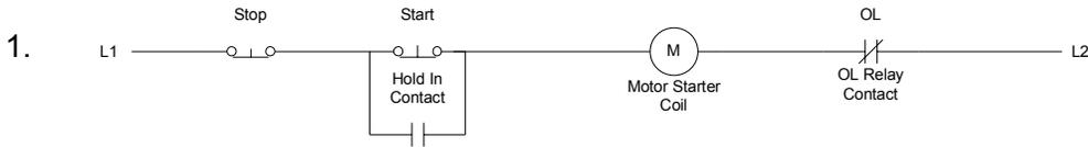
**1. Traditional 3 wire start stop motor control circuit with standard motor starter overload protection**
