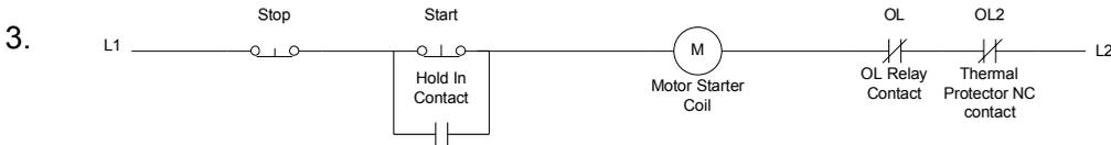
**3. Traditional 3 wire start stop motor control circuit with standard motor starter overload protection and motor internal thermal protector**
