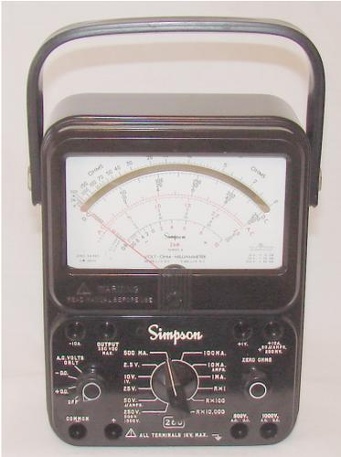
This had to be compared to the predecessor to the DMM, namely the Simpson 260 analog multi meter, which had an input sensitivity of  $5K\Omega$  per volt when measuring AC voltage. If we were measuring on the 250v scale then the input resistance would be  $5K \times 250 = 1.25 M\Omega$  and on the 50v scale it would be  $5K \times 50 = 250K\Omega$
