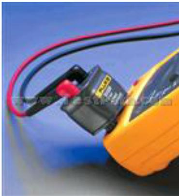
Fluke also sells an accessory that works for all their other meters, the Fluke SV225 part of the Fluke TL 225 stray voltage adapter test lead kit, that allows the same capability. On energized circuits the meter will indicate the real voltage and on non-energized circuits the meter will read close to zero, even if there are stray voltages.
