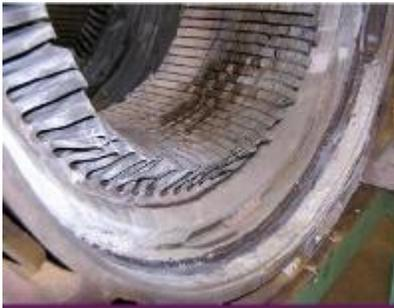
The picture to the left highlights this and shows in a dramatic way what happens when the rotor severely drags the lamination stack and produces a lot of damage.
