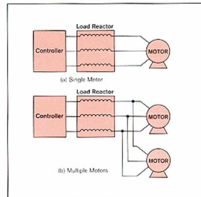
Figure 3. Typical Load Reactor Configuration
