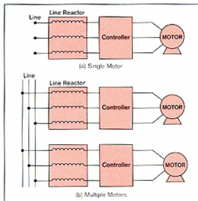
Figure 2. Typical Line Reactor Configuration
