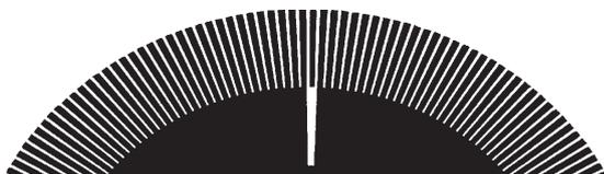
Absolute encoders provide a parallel output structure, the code of which gives a direct reading of the shaft's angular position, there is an optical reading device for each of the tracks. All disks are formatted with a Gray code; to ensure there are no reading errors, this code has only one bit change between divisions. E-PROMs inside the encoder are used to program the individual output code and add direction.
